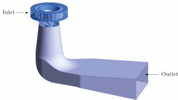
Figure 2. The computational domains, i.e., the guide vanes, the runner blades and the draft tube, and the boundary conditions.
