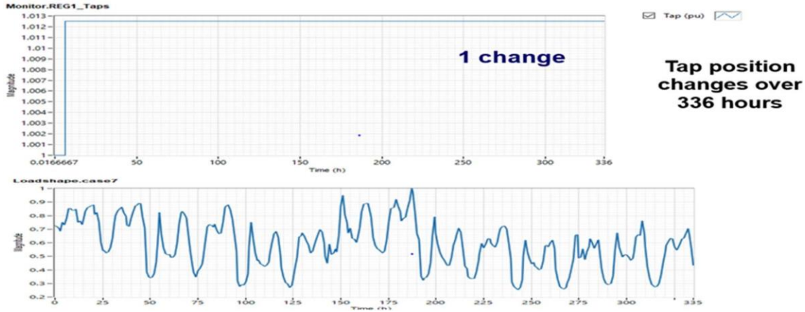
Fig. 3-8 OLTC operations for the VV function at 60% PV Penetration for the modified IEEE 37-bus system
