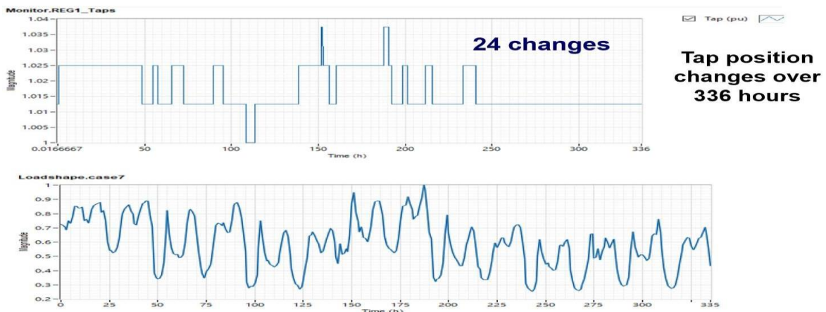
Fig. 3-13 OLTC operations for the FPF function at 60% PV penetration for Utility feeder
