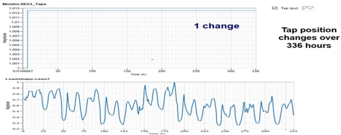
Fig. 3-9 OLTC operations for the VV function at 60% PV Penetration for Utility feeder
