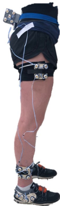
Figure 4.1 Participant instrumentation , where the shank, thigh, and pelvis marker clusters have been affixed to the lateral aspect of the IMUs while the foot cluster can be seen mounted to the posterior aspect of the shoe while the IMUs are located on the superior aspect of the shoe.
