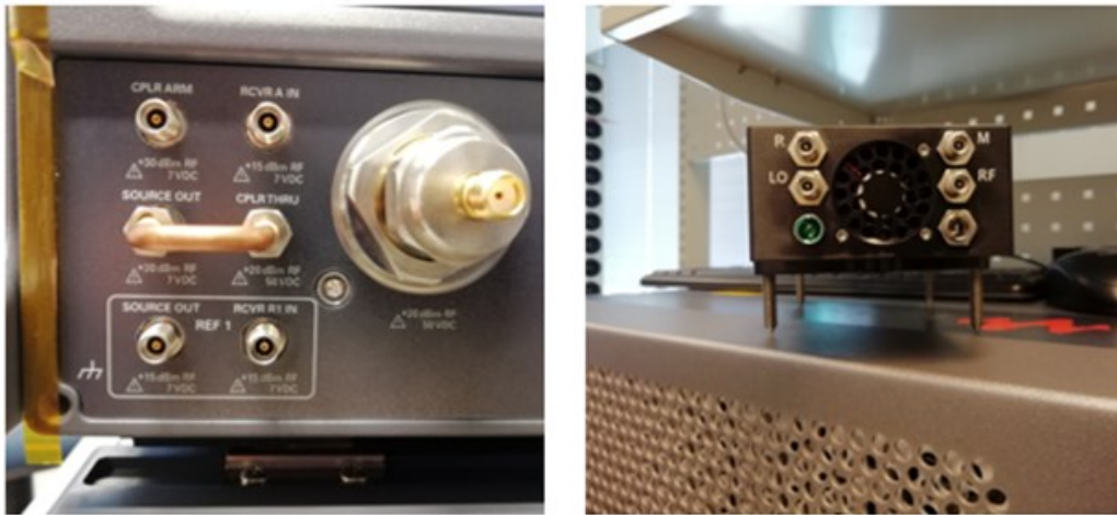
Figure 12. Front panel of PNA and TRX extender connection ports[18]
