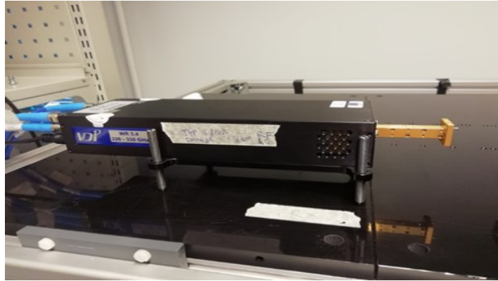
Figure 10. TRX frequency extender from VDI for 300 GHz application.
