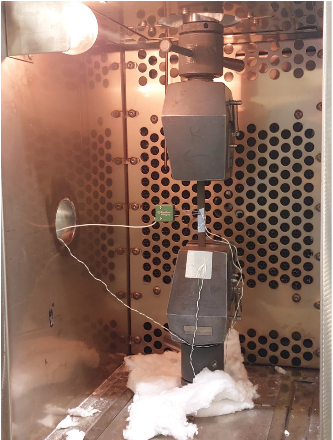
Figure 21 A sample placed in the load cell grips with the CMOD gauge and temperature probes attached, and their locations revealed by wires.
