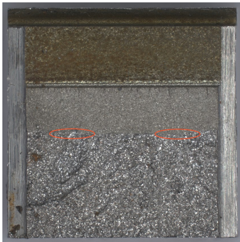
Figure 37 Common locations for crack initiation highlighted in orange.
