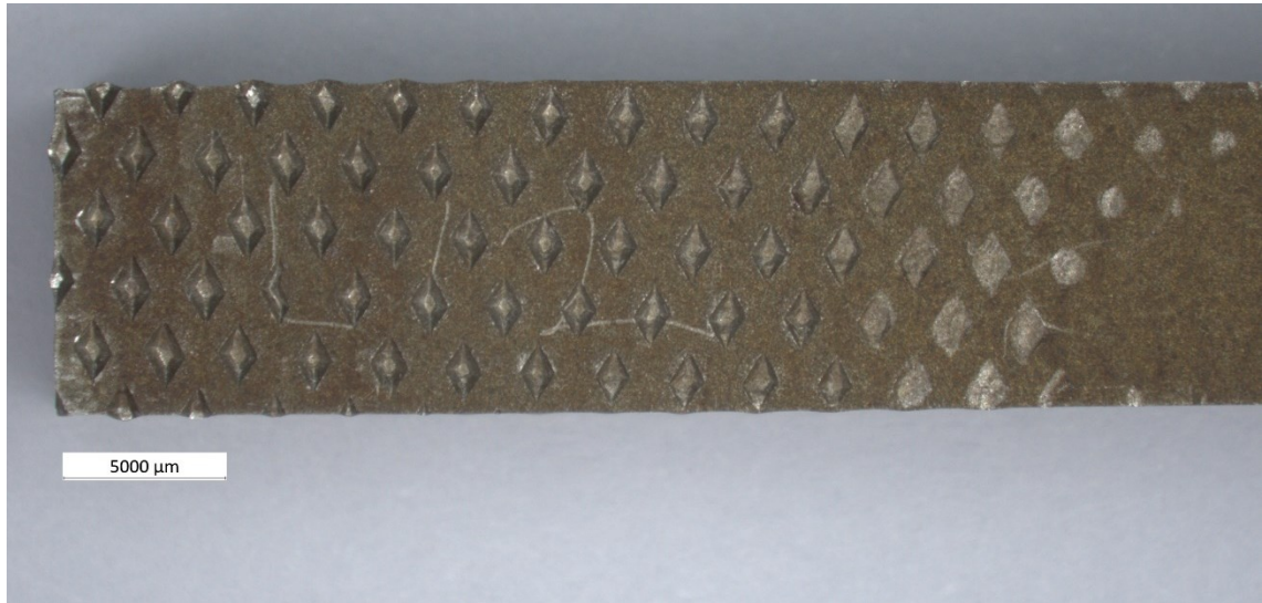
Figure 22 Roughing of the clamped region of the specimen to prevent slip.
