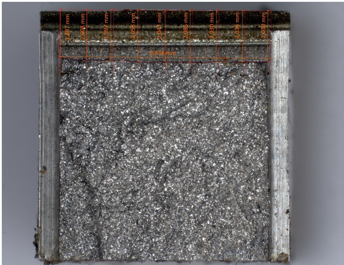
Figure 35 Fracture surface viewed and measured with a Zeiss AXIO Zoom V16.
