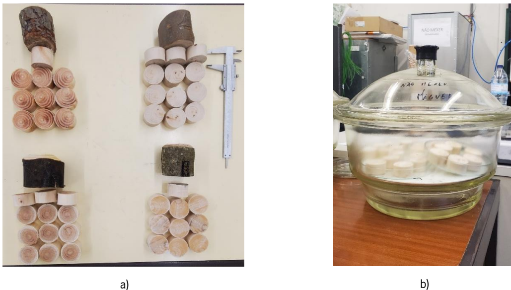
Figure 33: Samples prepared for the thermal properties determination experiment (a)) and the desiccator where the particles were stored (b)).
