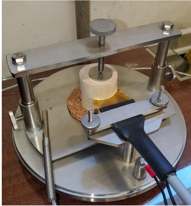
Figure 34: Experimental apparatus for the thermal properties determination.
