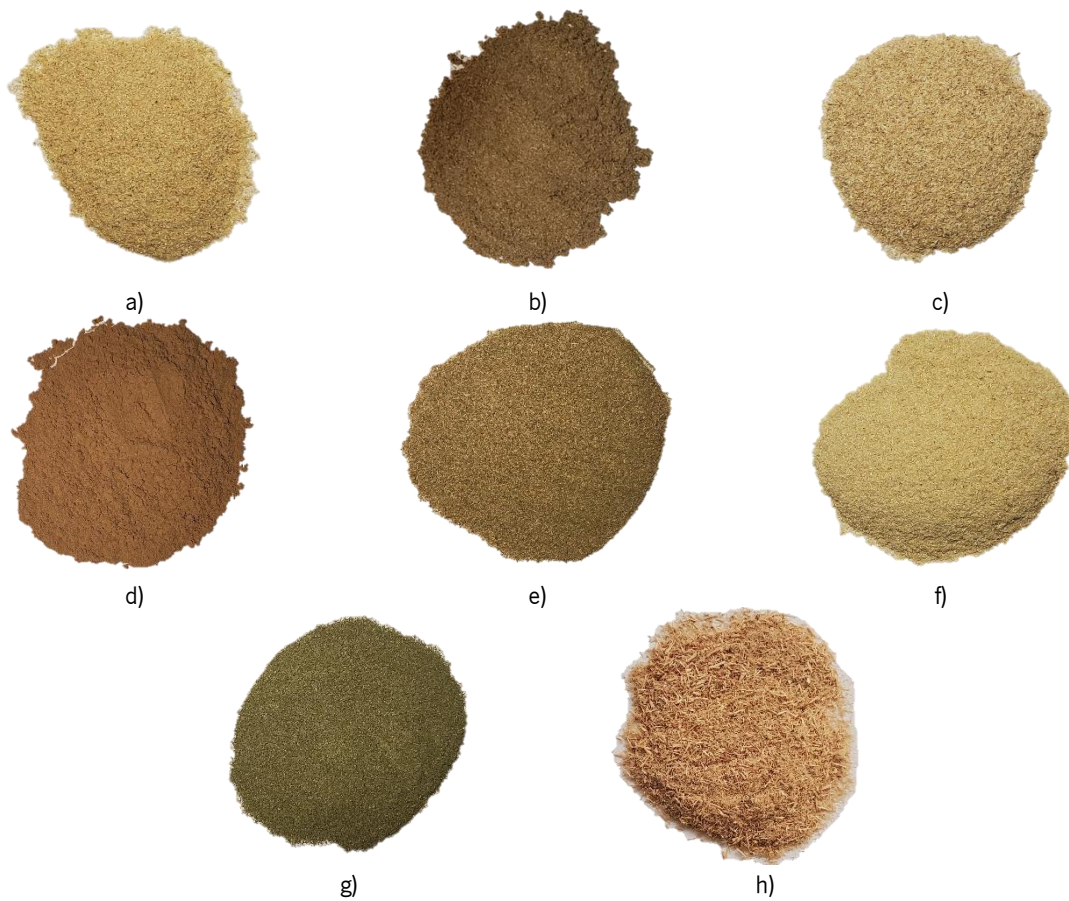
Figure 30: Samples used in the experiments: a) Pine trunk, b) Pine branches, c) Eucalyptus trunk, d) Eucalyptus bark, e) Eucalyptus branches, f) Acacia trunk, g) Acacia branches, and h) Olive branches.
