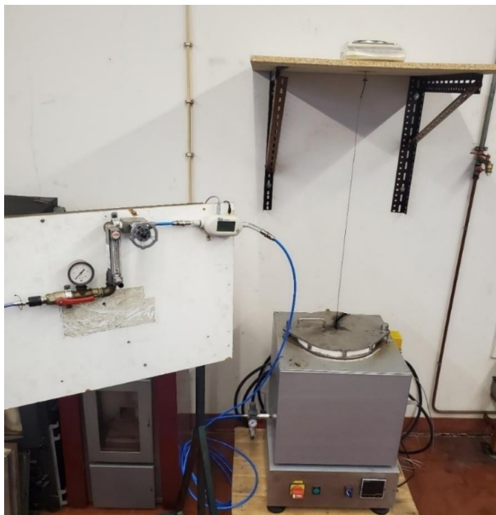
Figure 46: The small-scale reactor used for the macro thermogravimetric experiments.
