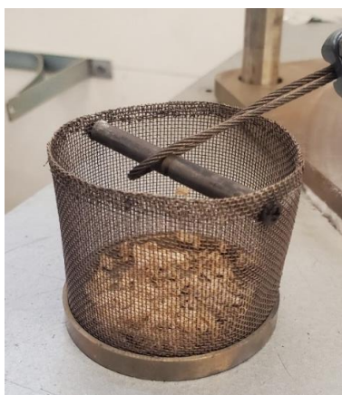
Figure 47: The basket where the biomass particles are introduced for the macro thermogravimetric experiments.
