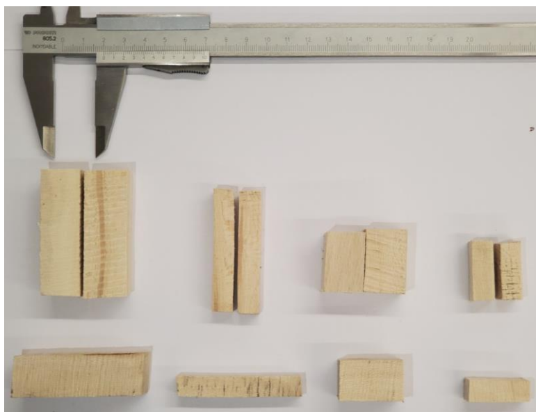
Figure 107: Particles produced to analyze the influence of different dimensions on the mass loss behavior.
