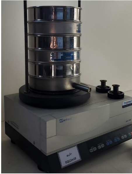
Figure 43: Vibratory sieve shaker and the sieves (8, 16, and 50 mm apertures) used to separate the particles according to their size.
