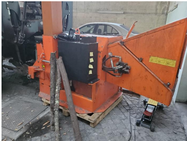
Figure 42: Knife chipper used to produce the woodchips.
