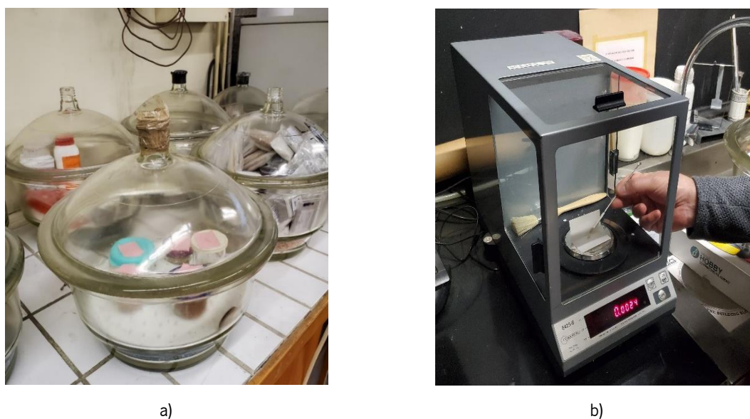
Figure 37: The different stages after the milling process of the raw materials: a) Storage in the desiccator, and b) weighing of the sample before the thermogravimetric experiment.
