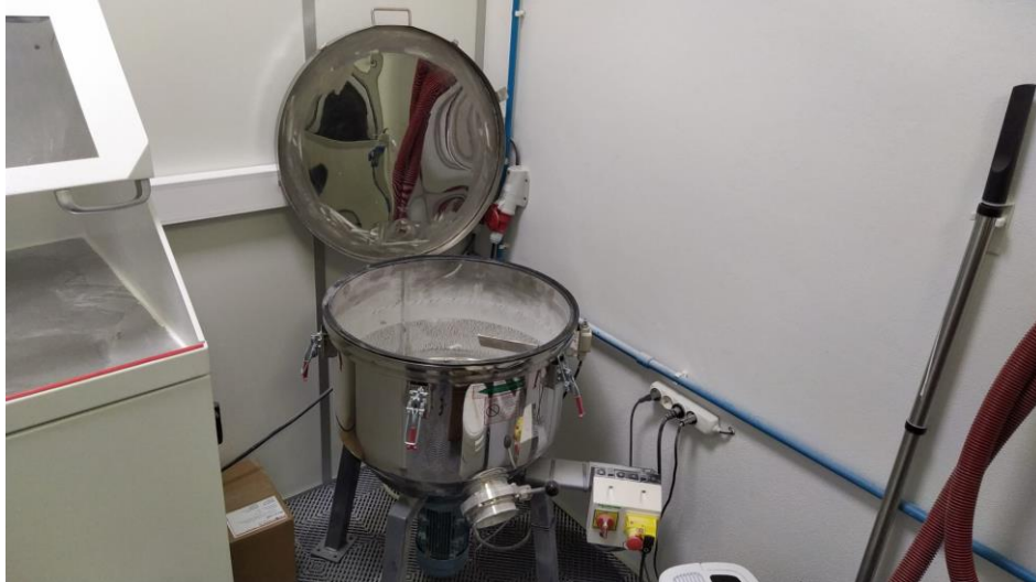
Figure 8 - Rotational mixer used for powder "mixture".
