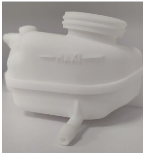
Figure 42 - Produced part with 100% virgin powder.
