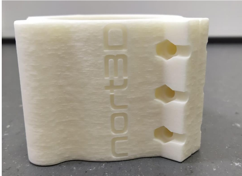
Figure 43 - Produced part with 100% reused powder with 12 reprocessing cycles.
