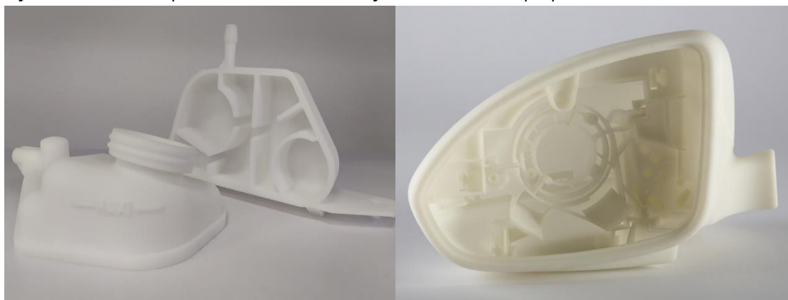
Figure 2 - Examples of PA12 printed parts by SLS
