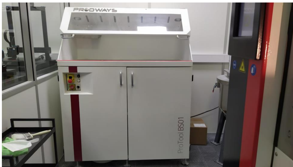
Figure 6 – Filtering machine used, ProTool BS01 .
