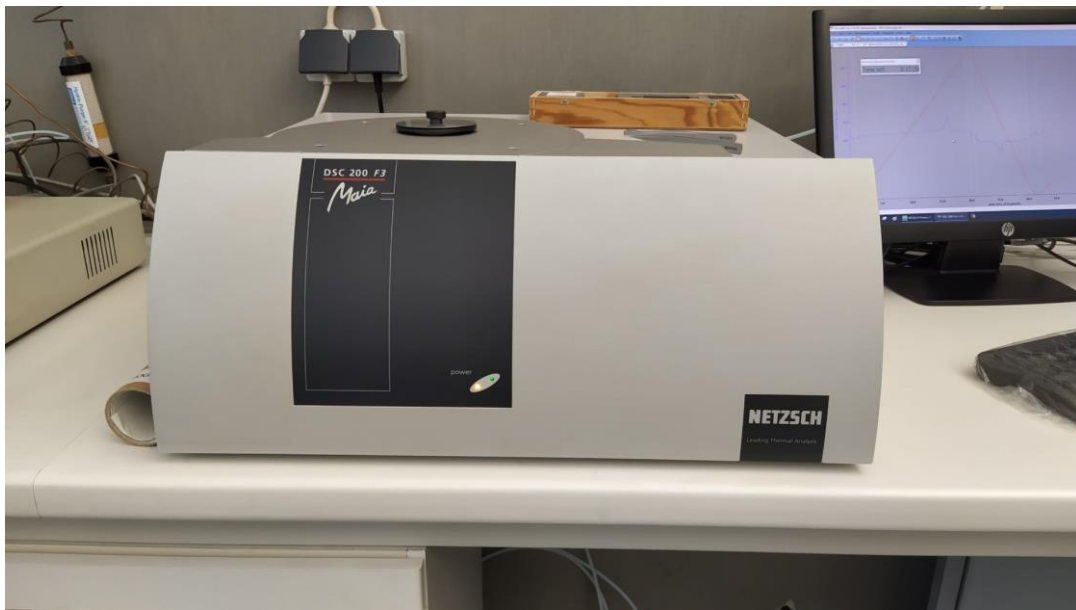
Figure 9 - DSC equipment used, NETZSCH DSC 200 F3 .
