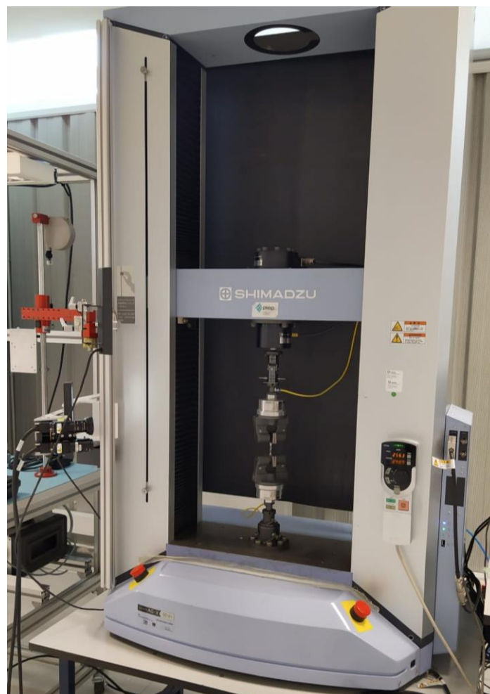
Figure 13 - Equipment used for tensile testing, Shimadzu AG-X with video extensometer.
