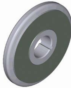
Figure 6 - Simplified tool like a shaped grinding wheel.
