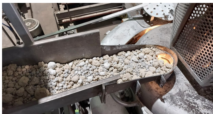
Figure 2. Feeding of the pelletized mixture to the furnace.
