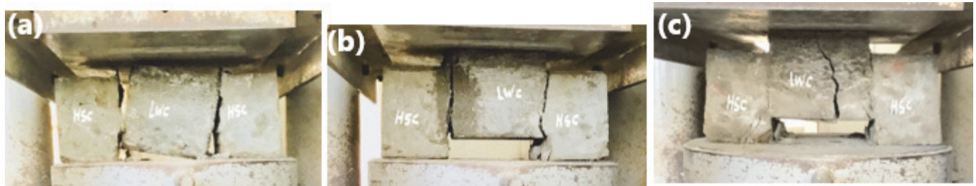
Figure 9: Mode of failure for push out test specimens; (a) triplets without connection method, (b) triplets with bond agent material, and (c) triplets with shear dowels.
