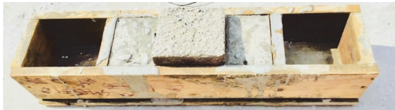
Figure 4: Casting triplet specimen for bond strength test.
