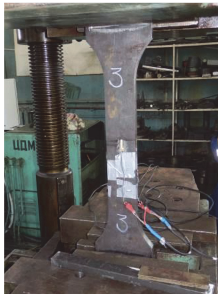
Figure 2: Tests of a corset specimen cut from the I-beam flange
