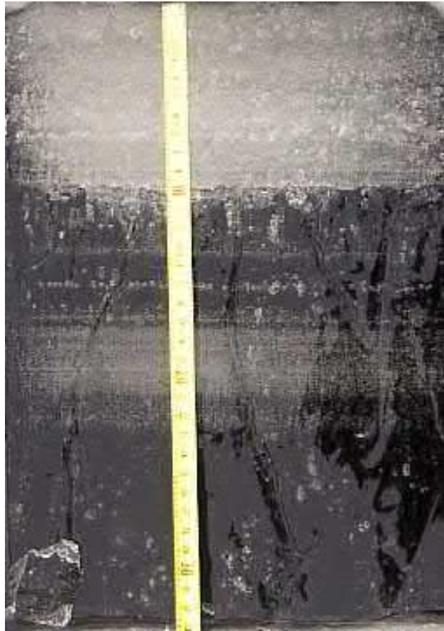
Figure 5.8: Layered structure of lake ice. Ice thickness is 33 cm, of which the upper 10 cm is opaque snow-ice and the lower 23 cm is clear congelation ice. Congelation ice also shows some layers of gas bubbles. Photo: Matti Leppäranta.
