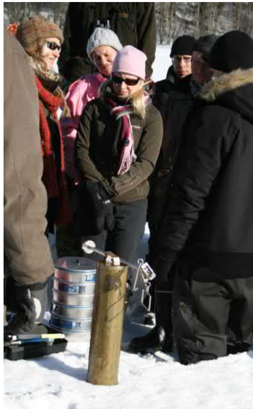
Figure 4.19: Measuring water equivalent of snow with a cylinder and steelyard. If the thickness of the snow cover is also measured, mean density of the snow pack is acquired. Pictured are students on the course 'Geophysics of snow and ice' at Lammi Biological Station. Photo: Matti Leppäranta.
