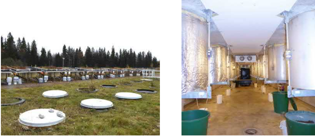
Figure 4.14: Soilia lysimeter field in Lahti. The foreground of the left image is covered by active lysimeters. The photo on the right depicts underground lysimeter containers under the field. Photos: Leena Leppäranta.
