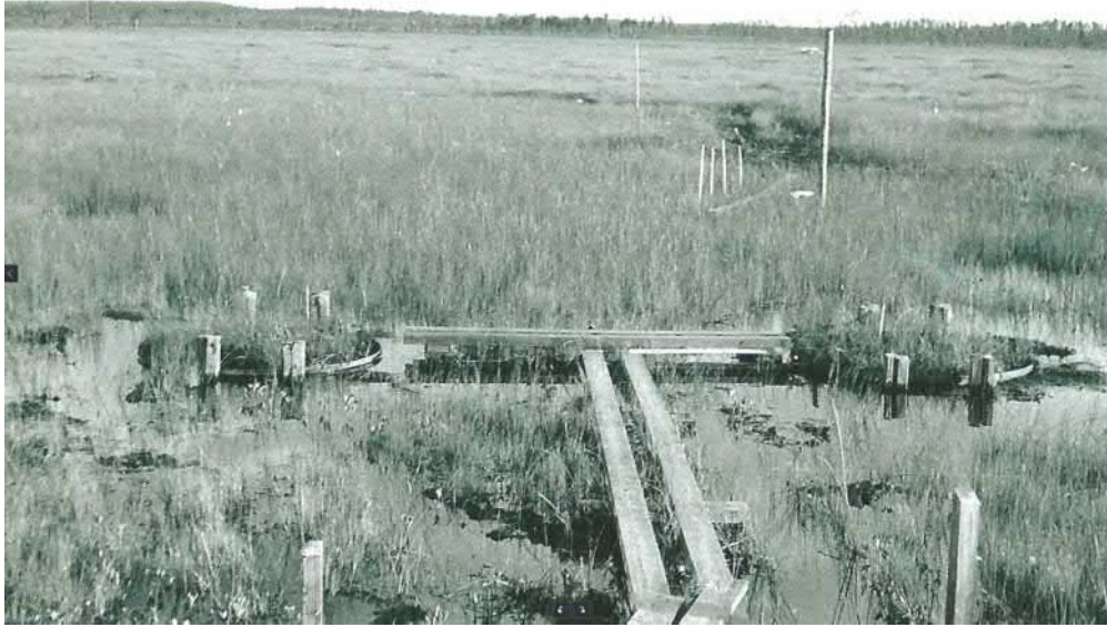
Figure 4.13: Measuring evaporation over Möksy fen (South Ostrobothnia, Finland) using a lysimeter. Photo: Courtesy of Juhani Virta.
