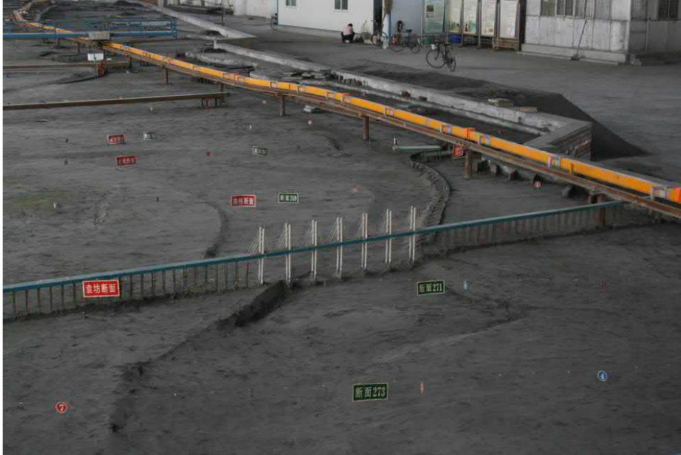
Figure 2.12: In the flow of rivers, shallow water waves play a dominant role in the dynamics. Therefore, its effects can be studied with a physical model. Pictured is a 1 km long model of a section of the Yellow River. Photo: Matti Leppäranta.
