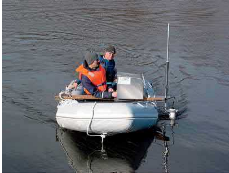
Figure 6.9: The most significant innovation in measuring flow velocity since the propeller current meter has been the Acoustic Doppler Current Profiler (ADCP). In Finland this method was adopted in 1994, and it has made the measurement of large discharge values significantly easier. Photo: SYKE (Kuusisto, 2008).
