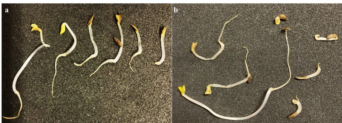
Figure 8: Phytotoxicity experiments: (a) in RR-141 solution, (b) tap water.
