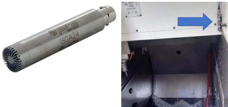
Figure 23 – PCB a30A24 microphone and its installation.
