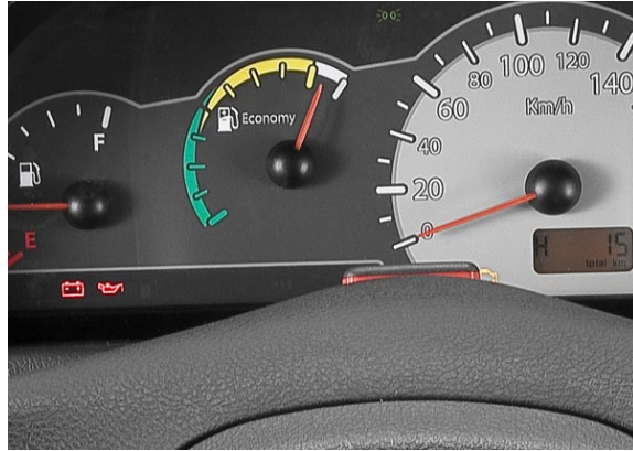
Figure 41 – Indicator of fuel economy in the instrumentation panel of a passenger vehicle. Adapted from (SANDOVAL, 2008)
