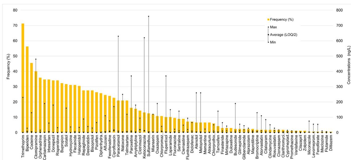
Fig. 2. Frequency of occurrence (yellow bar) and minimum, average, and maximum concentrations (black point-line) of quantified pharmaceuticals present within the samples. (For interpretation of the colour in this figure legend, the reader is referred to the Web version of this article.)
