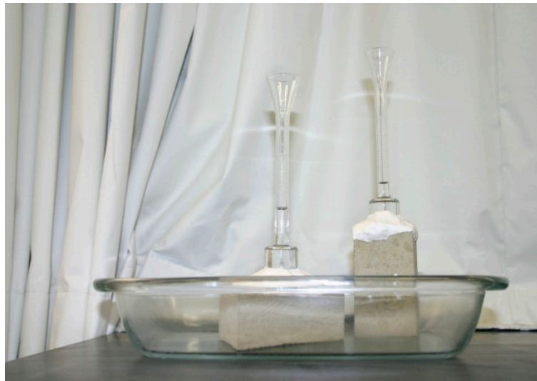
Figure 4. Testing equipment for the absorption of water under low pressure: Karsten glass pipe on sandstone samples inside a glass tray.
