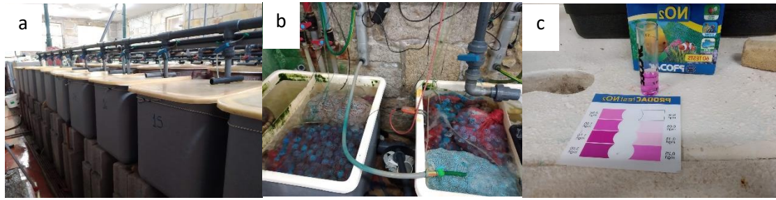
Figure 10: Thermoregulated water recirculation system. a) – fiberglass tanks of 100L water-capacity; b) – biological filter; c) – PRODACTestkit.
