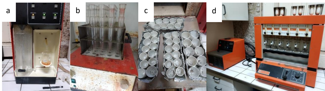
Figure 12: Apparatus for proximate composition analyses. a), b) – Kjeldahl system for crude protein content; c) – crucibles for humidity and ash content; d) – Soxtec systems for crude lipid content.
