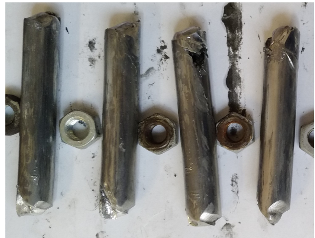
Figure 2: Photographs taken on the capsules (a) before and (b) after the ECAP deformation.
