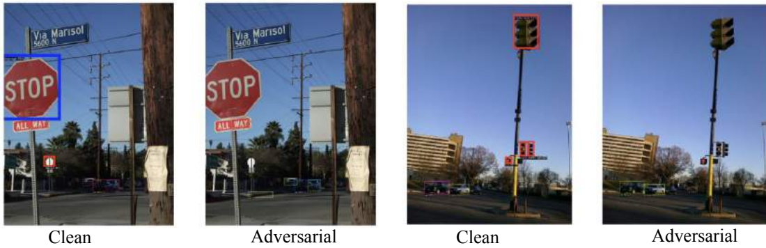
Figure 4: Traffic light detection for clean and adversarially perturbed inputs [125]. For humans both images still look the same however a neural network fails to detect traffic signs, which can lead to serious consequences. Therefore, we focus on making our classification systems robust against adversarial perturbations.
