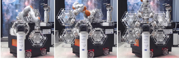
Fig. 8. Single, double and triple mating connections during the dPAMT demonstration.
