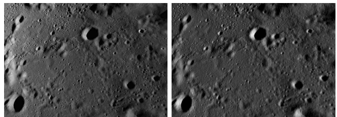
Figure 12. The left image is a cropped and rectified photograph taken by the SpaceIL Beresheet Lander. The camera's pose and intrinsic parameters were obtained from a single image, using crater landmarks detected by [38]. The right image is a corresponding image rendered with CosmoScout VR using LOLA elevation data. While the geometric similarities are apparent, quantitative image comparisons are future work.
