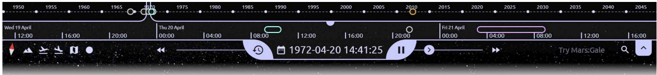
Figure 7. A central element of CosmoScout’s user interface is an interactive timeline. The upper overview-timeline is usually hidden and can be expanded by clicking the arrow-button on the right-hand side. This overview can be dragged and zoomed independently of the main timeline at the bottom. Temporal events are shown with colored circles or bars. The simulation speed can be adjusted with the slider below the timeline.
