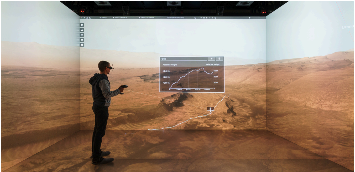
Figure 1. Exploring Gale Crater on Mars: Interactive visualization of HiRISE data from the Mars Reconnaissance Orbiter using 28 projectors of the aixCAVE at RWTH Aachen.
