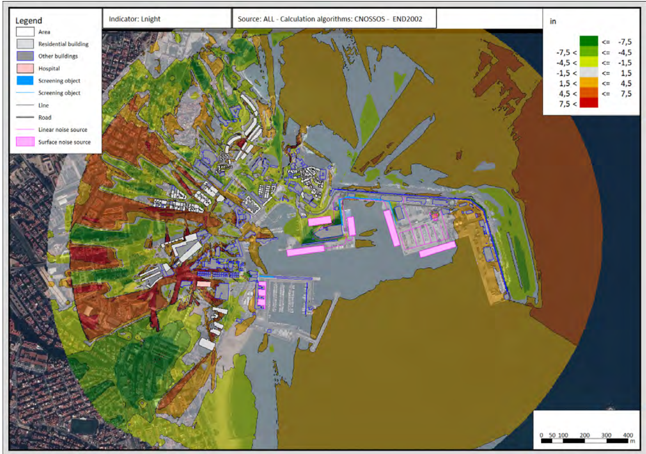
Figure A6: Difference between L_{night} estimation with 2015/996 algorithm and the one of the old Annex II of the END
