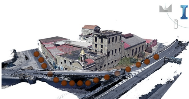
Figure 6. Detail of the 3D model obtained with SfM algorithms applied to spherical images acquired by rapid mapping techniques (in red the acquisition points).
