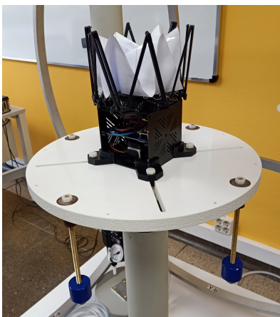
(a) CubeSat attached to air bearing system right view.
