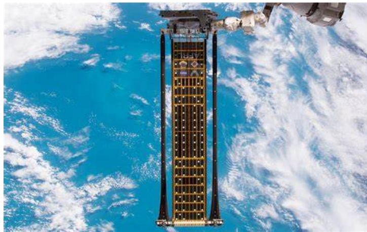
Figure 2.7 Roll Out Solar Array (ROSA) structure. Source: [15]
