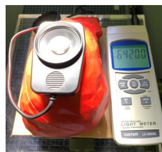
Figure 5. Digital data logger illuminance meter LX-2000SD.
