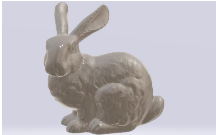
Figure 12. The Stanford bunny mesh model built of 69 630 watertight triangles.
