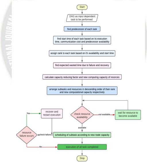
Figure 2. Flowchart for DAG based Reliable Scheduling Approach
