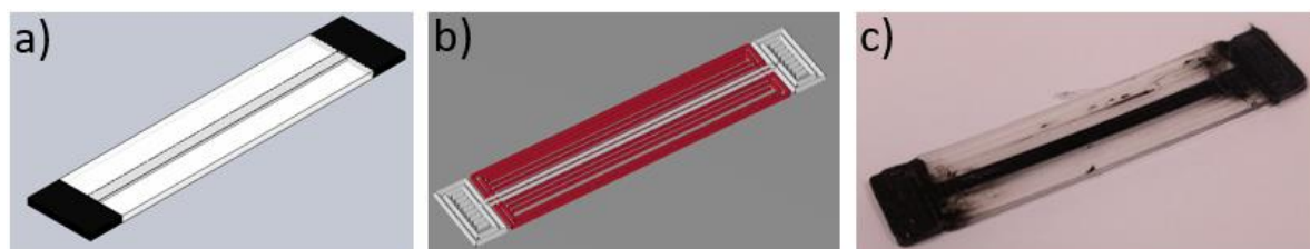
Figure 3. Design-to-fabrication process: (a) generating CAD model; (b) rendering code for 3D printing; and (c) resulting physical sensor.
