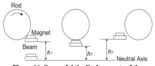
Figure 16: Successful tip displacements of the piezoelectric beam.
