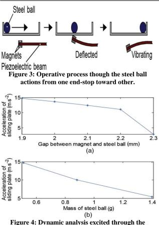
Figure 4: Dynamic analysis excited through the slider: smallest outside acceleration required toward release. the steel ball from the magnets.
