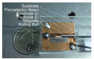
Figure 13: Experimental model of the piezoelectric pulse generator.
