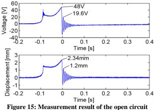
Figure 15: Measurement result of the open circuit voltage and tip displacement of the piezoelectric beam.
