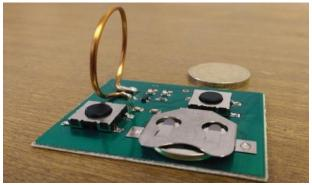
Figure 19: Testing set-up of the Colpitts oscillator.
