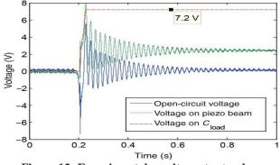
Figure 12: Experimental results: output pulses generated with and without prebiased piezoelectric beam.
