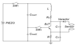
Figure 22: Transmitter aimed at the piezoelectric generator schematic of the FM.
