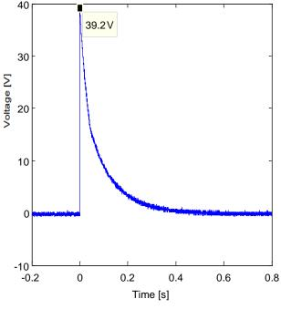
Figure 17: Output measurement of the pulse generator with a 1 M $\Omega$  load.
