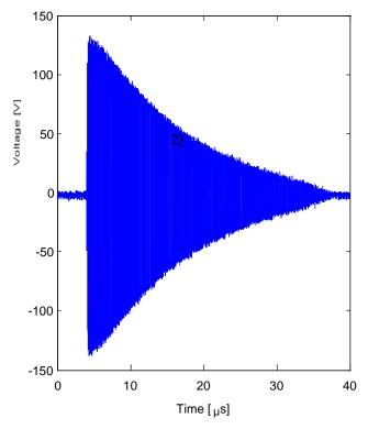
Figure 20: Transient measurement of the received signal for one operating cycle. The transmission distance is ~ 5 cm.
