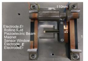
Figure 14: Rolling rod generator of the experimental set-up.
