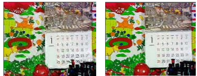
Figure 7 - Mobile&Calendar (frame 33) scaled at QCIF resolution at 256Kbps. Left IB-MCTF-1. Right IB-MCTF-2
