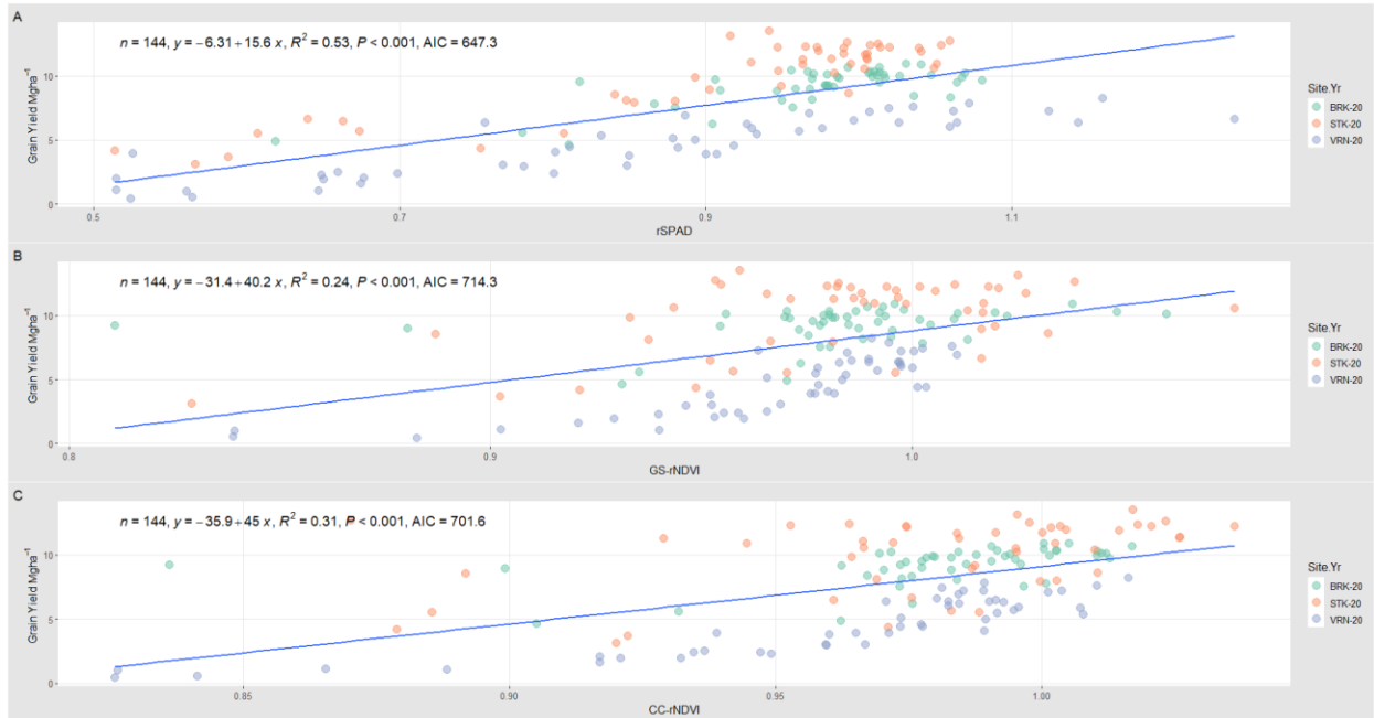
Figure 2.2 Sensor comparison between the relative VI values for the SPAD (A), GreenSeeker (B), and Crop Circle sensors (C) at the VT stage. The population for each equation is represented by n , the equation is represented by y , the coefficient of determination is represented by R^2 , the P-value by P , and the Akaike Information Criterion by AIC
