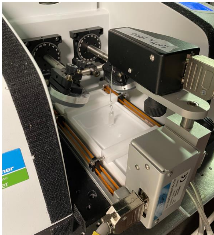
Figure 4. Experimental setup featuring Langmuir trough, barriers, Wilhelmy plate, FTIR spectrometer, and mirrors
