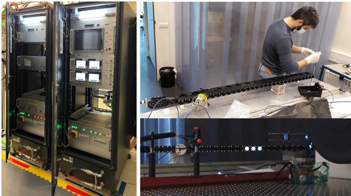
Figure 6. Left ) The two main electronic cabinets of the Hardware Facility Control System that will be installed next to the telescope yoke on the Azimuth floor. Right ) Integration (top) and illumination test (bottom) of the Calibration System illumination units. Even though all 30 integrating spheres are illuminated, because their outputs are near collimated beams through their lenses in front, only 3 beams are seen.
