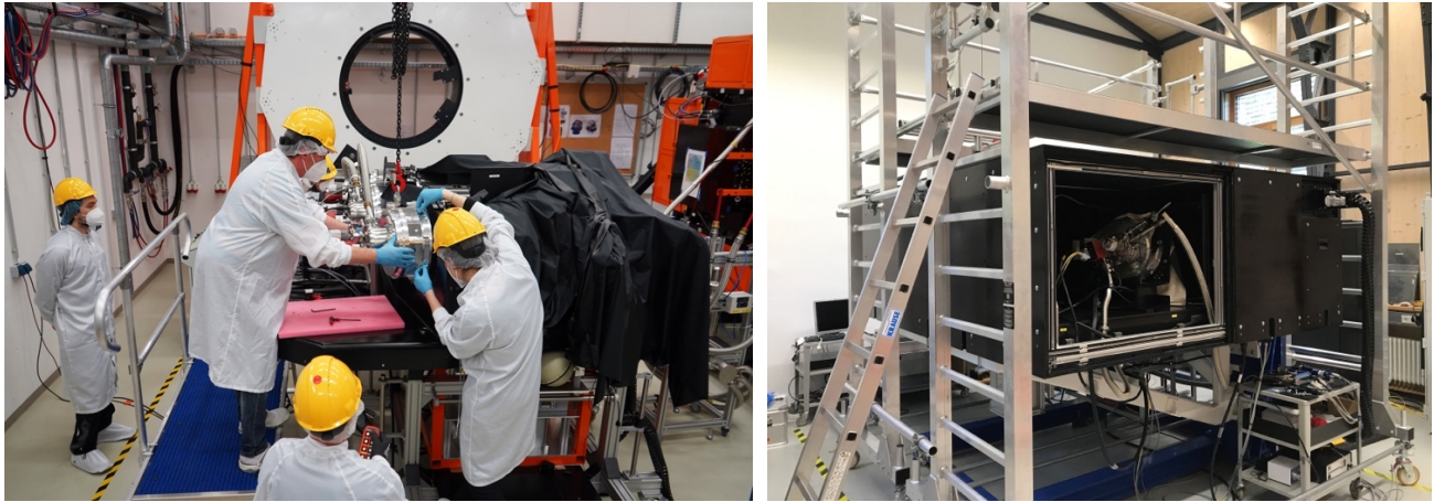
Figure 5. Left ) Reintegration of the first Low-Resolution Spectrograph in Potsdam after delivery from CRAL. One of the detector systems is being installed. Right ) The High-Resolution Spectrograph during Local Acceptance Review inspection in Heidelberg. The black panels are part of the thermally insulated spectrograph cover. One panel has been removed for inspection of one of the CCDs. The aluminium scaffolding surrounding the HRS is used to provide the same access conditions to the slit unit as at the telescope by means of an access port on the top reached from the observing floor.
