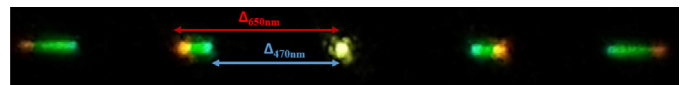
Fig. 4. Diffraction pattern of a sample-flied, structured with a line distance d_{hatch} = 40 μm, illuminated with the wavelength range \lambda = 470 nm – 650 nm.
