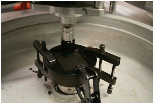
Figure 4. Experimental set-up during the polishing correction technique showing the flat polishing tool, the additional adapter and the polishing suspension.
