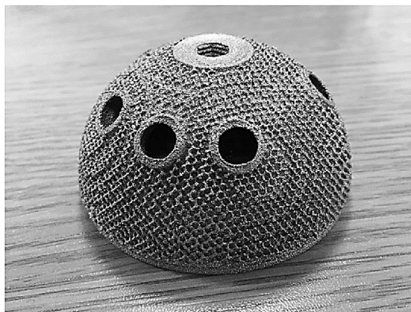
Figure 3.7. Acetabular cup produced by Additive manufacturing [247]
