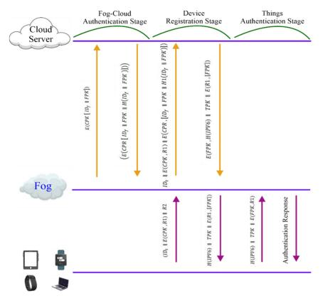
Figure 3. Flowchart of the planned authentication mechanism.
