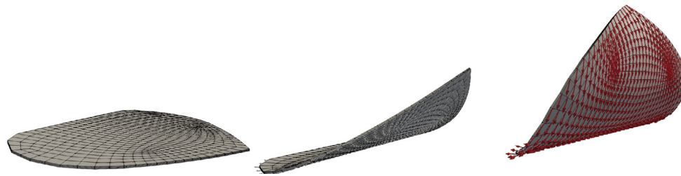
FIGURE 9 Deformed flower petal due to an electric field in X-direction at different electric field intensities. (Left) Resulting deformation at 0.14 V. (Middle) Deformation at 0.72 V. (Right) Deformation at 1.44 V. The color map refers to the displacement magnitude.
