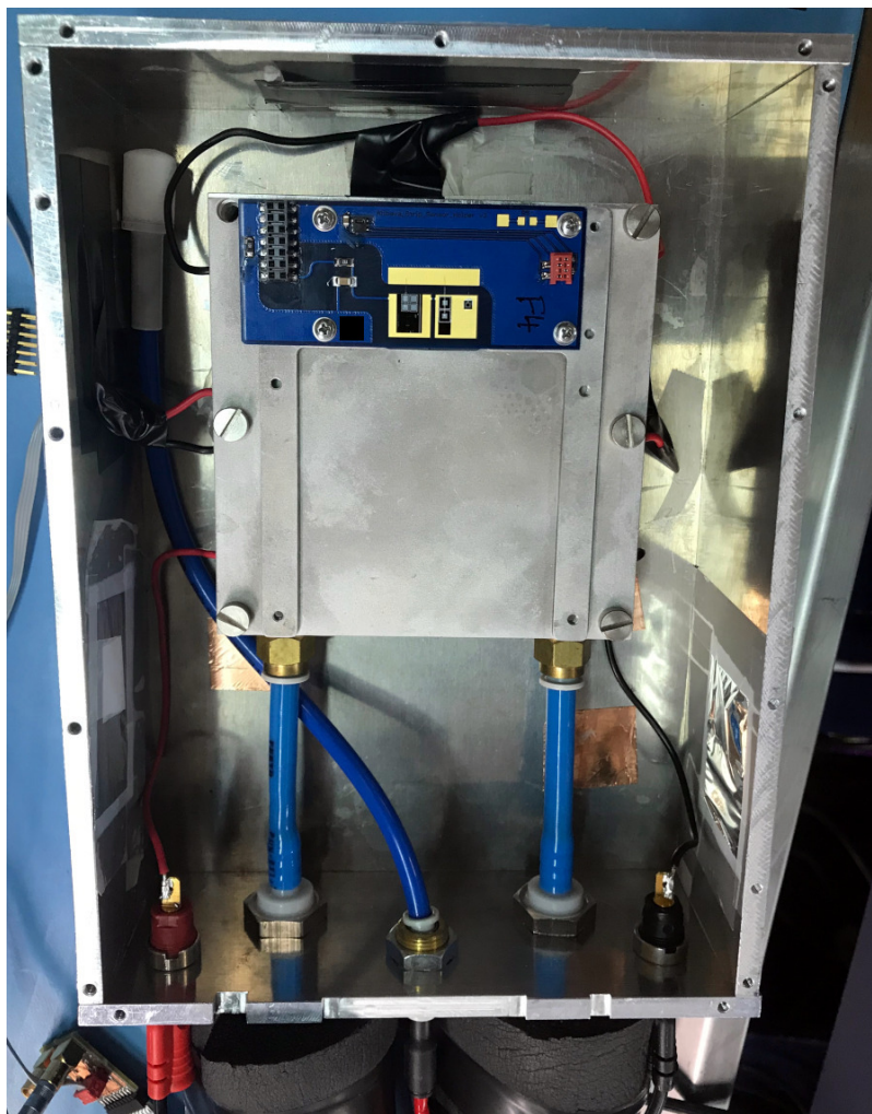
Figure 4. Setup for AREA-X measurements: the sensor test PCB is mounted on an aluminium holder plate for easy exchange.
