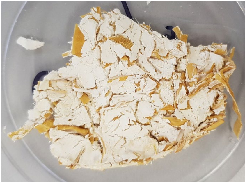
Figure 18. 20% short rau pressed ACC sample made early in the project to investigate bonding.
