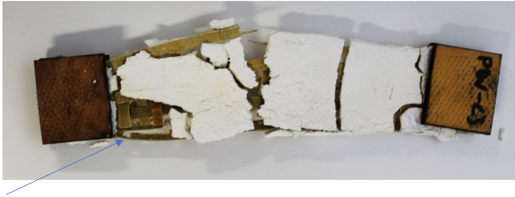
Figure 27. PW-C3, a plain weave ACC after break. Blue arrow indicates split at the base of the rau .
