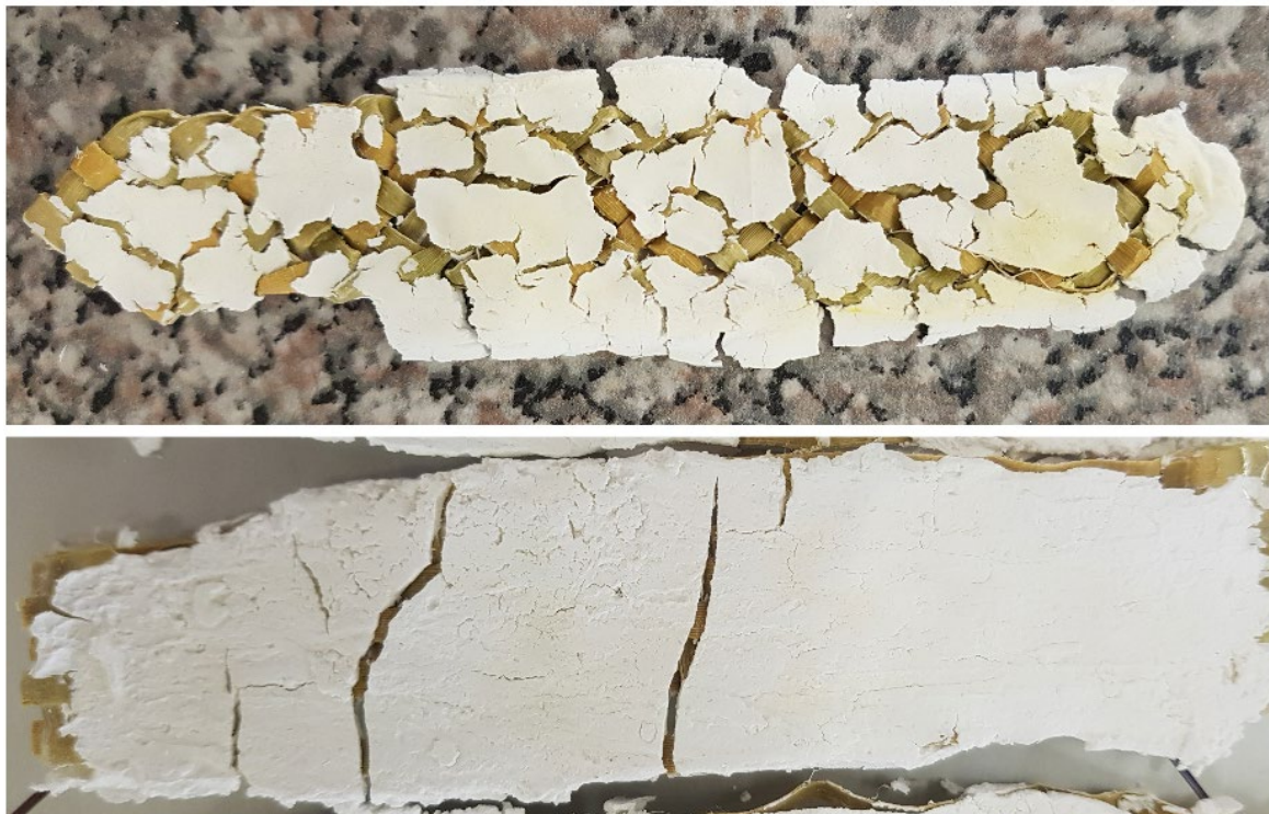
Figure 20. Comparison between 20 wt.% cellulose matrix cracks after drying via oven (top) and 25 wt.% matrix cracks after freeze drying (bottom).
