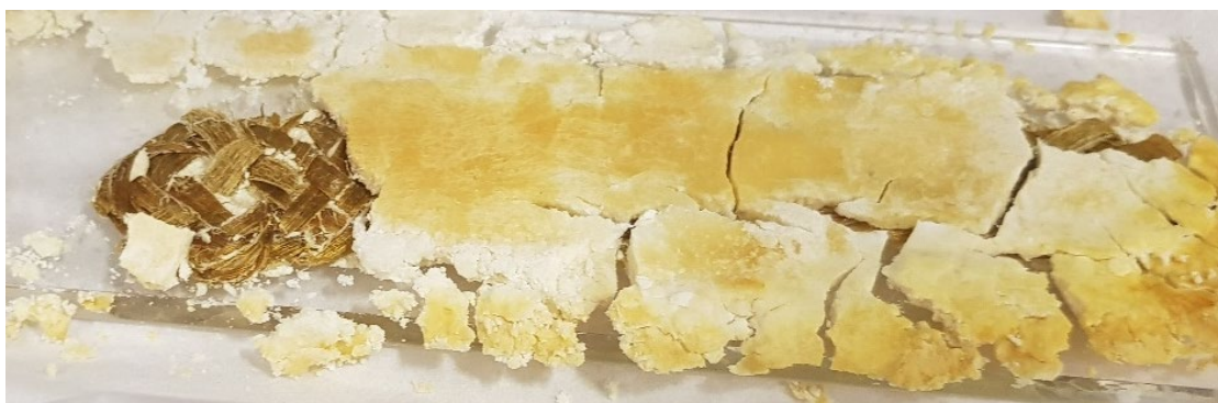
Figure 19. A 25 wt.% ACC sample which has cracked during the gelling phase. The harakeke rau can be seen to have already dried out despite the gel being moist. The brown colour in the cellulose matrix is due to it not having been washed yet, which happens after gelling.
