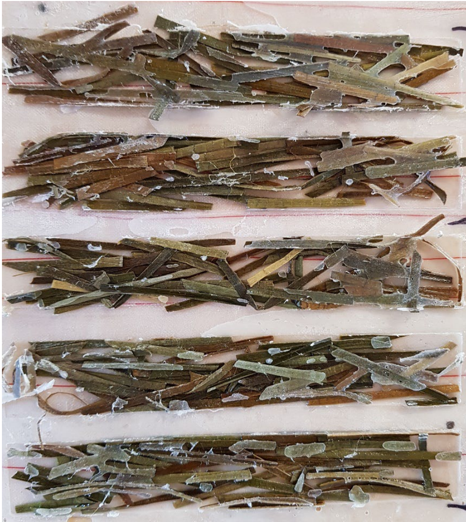
Figure 17. Experimenting with the bonding between pre-treated rau and epoxy.
