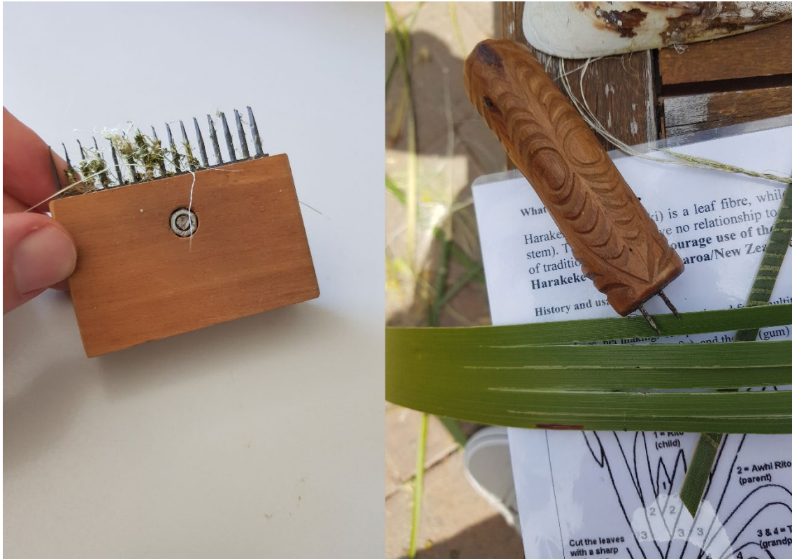
Figure 11. A custom hae hae tool made for this research project based on a shearing comb hae hae used by Kerepeti Paraone (left) and Reihana Parata's hae hae (right).
