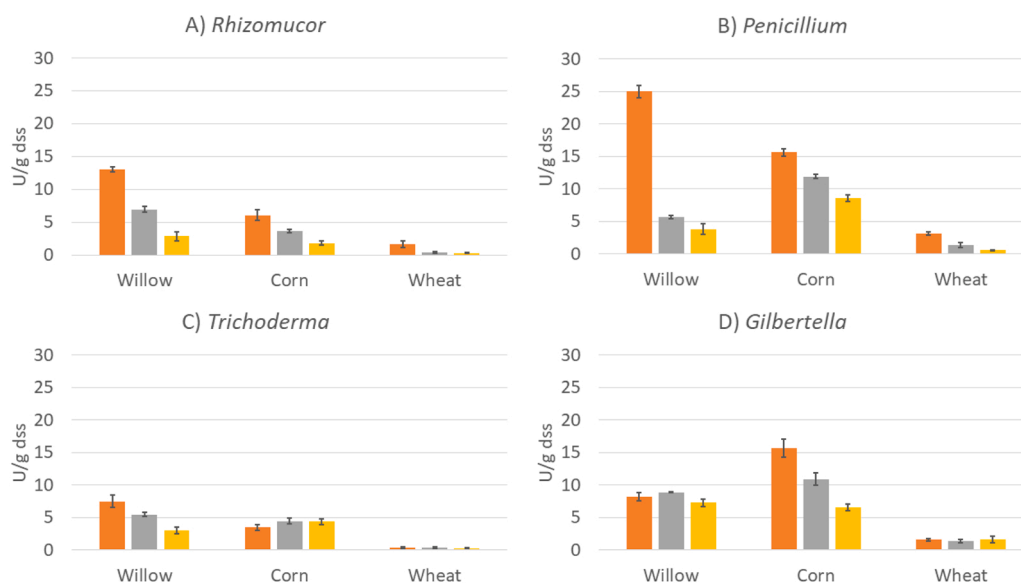
Fig. 1. \beta -glucosidase activities of the fungi on willow wood chip, dry corn stover and wheat straw substrates: R. miehei (A); P. aurantiogriseum (B); T. reesei (C); G. persicaria (D). Orange: on day 3; grey: on day 6; yellow: on day 9.
