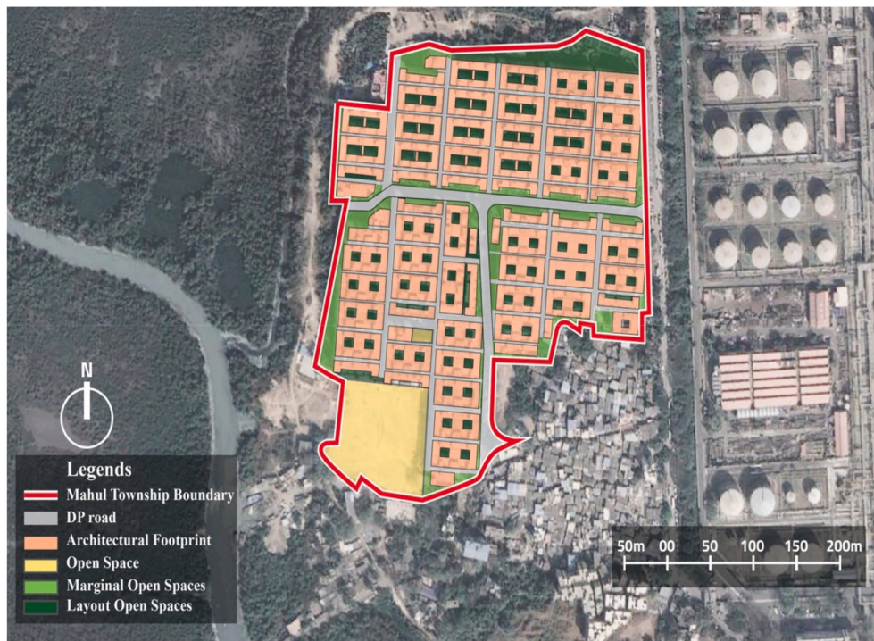
Fig. 2. In Mahul, the architectural footprint dominates the land-plot. Densely packed buildings and restricted open space prevent ventilation and sunlight. Source: Google Earth image modified by Author; inspired by Indorewala and Wagh (2017).
