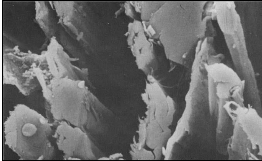
Figure 8.3 Transverse sections of hemp fibres. These fibres are thicker than the nettle and flax fibres and have narrower lumina. As the hemp lumen are narrower and indistinct, this image was not used in the subsequent analysis of lumen/cell diameter ratios. (Ryder and Gabra-Sanders 1987).
