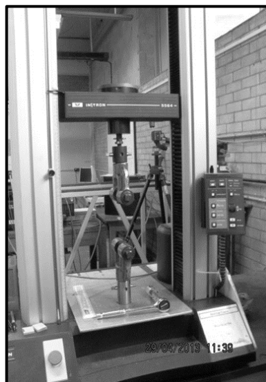
Figure 6.2 5564 Mechanical stress/strain testing equipment (Instron High Wycombe UK 2016)
