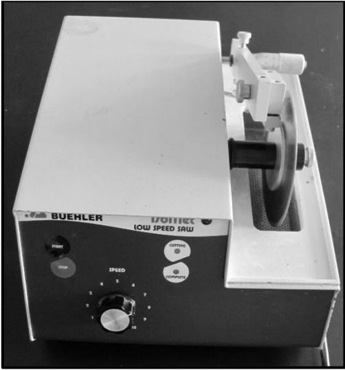
Figure 8.12 Buehler Isomet Low-Speed Rotary Microtome. Used for the cutting of 1-2mm thick sections from the 6mm diameter epoxy resin mould. The cutting wheel used was a 5ins. diameter diamond wafering blade.
