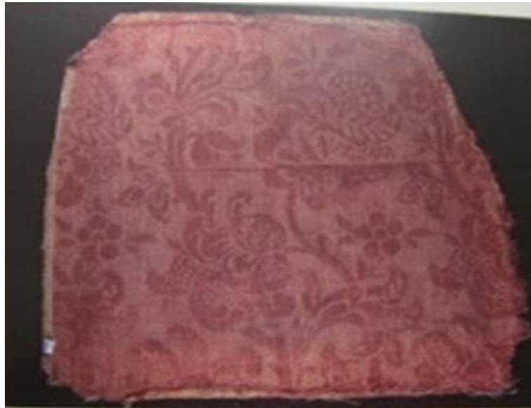
Figure 12.1.1. RW 337. A 19 th . Century seat cover (Ginsberg Catalogue No. 154). Late 19 th -century cotton and bast furnishing of Brocatelle weave. 46.3 x 57.1 cm. Cotton warp ends 12/cm Z twist (average dia. 0.64mm). Bast fibre weft picks 28/cm 2ply Z twist (average dia.0.8mm).
