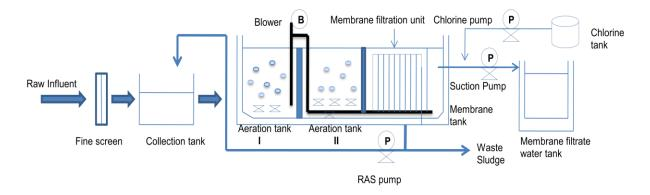
Figure 1: Schematic Diagram of the hospital wastewater treatment plant
