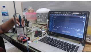
FIGURE 1 . Front View Module with experiments on a fetal heart rate simulator
