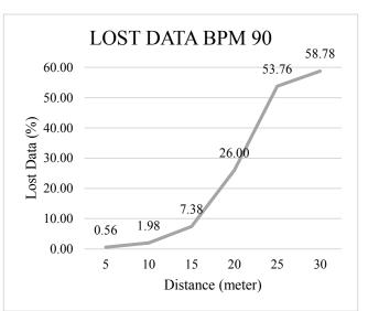
FIGURE 4 . Experiment using a fetal heart rate simulator at the Lost Data BPM setting of 90
