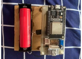
FIGURE 2 . Design Modul and Overall Circuit Design in Research on Fetal Heart Rate with ESP32
