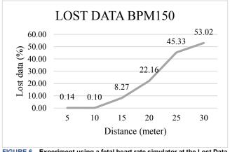
FIGURE 6 . Experiment using a fetal heart rate simulator at the Lost Data BPM setting of 150
