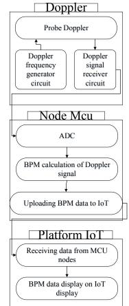
FIGURE 1. The System Block Diagram in Research Fetal Heart Rate
