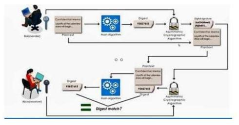
Figure 1: Block Diagram of a Digital Signature
