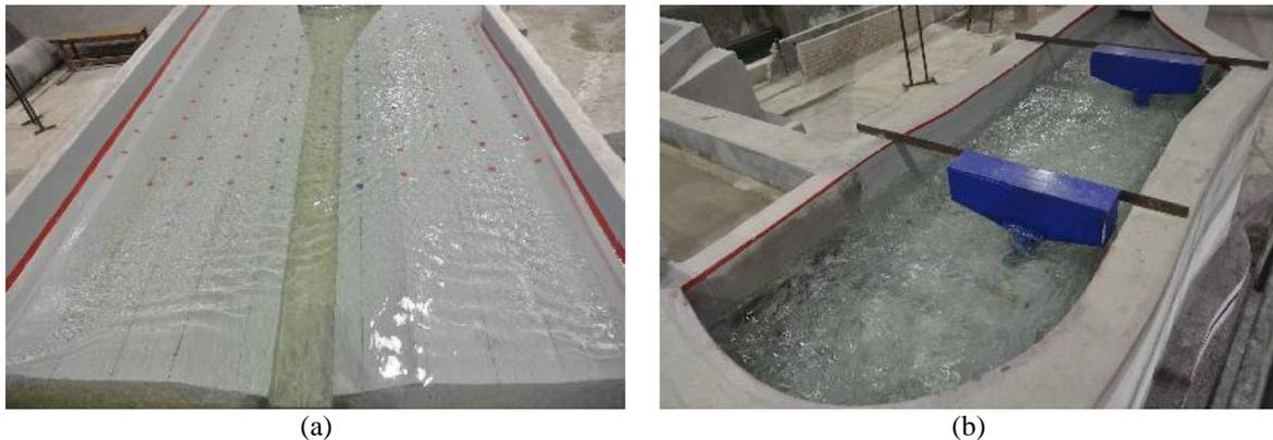
**Fig. 5 - Flow at discharge of 121 L/s at at (a) Sungai Bunus, and; (b) stilling basin (with piers)**
