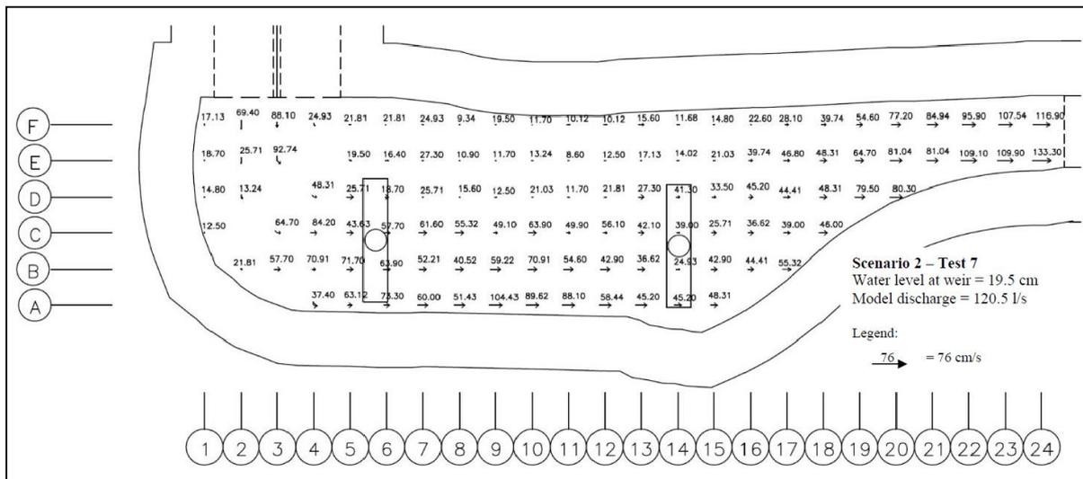
**Fig. 12 - Stilling basin velocity distribution maps for 121 L/s (with piers)**
