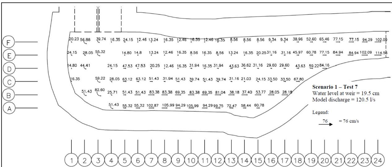
**Fig. 9 - Stilling basin velocity distribution maps for 121 L/s (without piers)**
