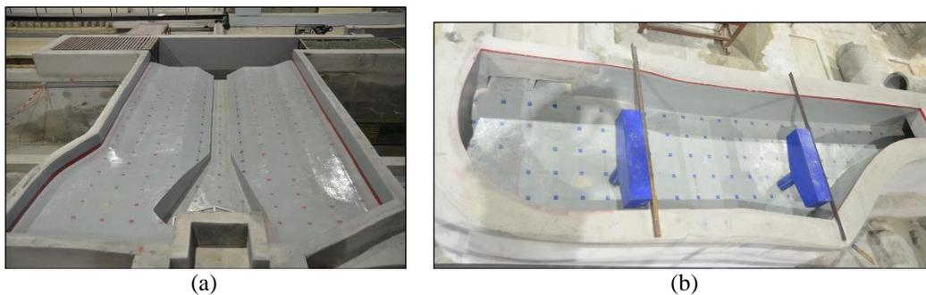
**Fig. 3 - Data collection points grid mesh at (a) Sungai Bunus, and; (b) stilling basin**
