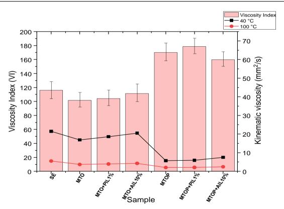
Fig. 4 - Graph of kinematic viscosity and viscosity index
