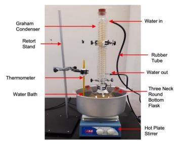
Fig. 2 - Degumming process setup
