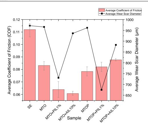
Fig. 5 - Graph of average coefficient of friction (COF) and average wear scar diameter (WSD)
