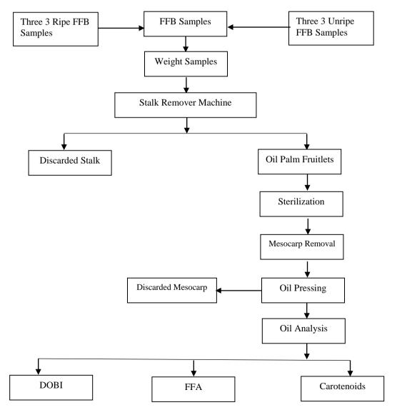
Fig. 3 - Flowchart for process study methodology
